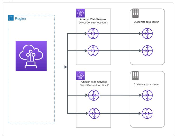
The following procedures demonstrate how to use the AWS Direct Connect Resiliency Toolkit to configure a maximum resiliency model.
