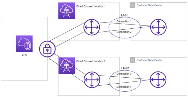
You can create a LAG from existing connections, or you can provision new connections. After you've created the LAG, you can associate existing connections (whether standalone or part of another LAG) with the LAG.
