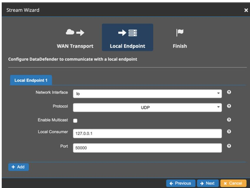
The screenshot shows the 'Stream Wizard' interface in the 'Local Endpoint' step. At the top, there are three tabs: 'WAN Transport', 'Local Endpoint' (selected), and 'Finish'. Below the tabs, the text reads 'Configure DataDefender to communicate with a local endpoint'. The form contains the following fields:
