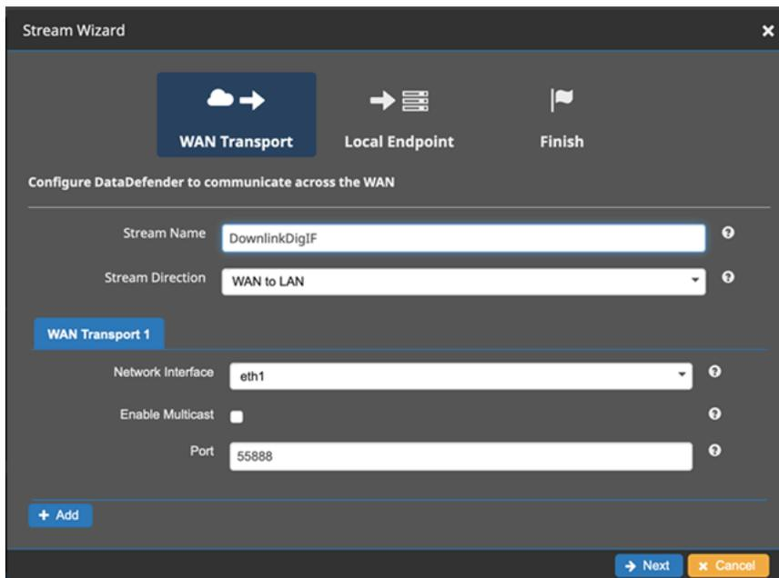
The screenshot shows the 'Stream Wizard' interface in the 'WAN Transport' step. At the top, there are three tabs: 'WAN Transport' (selected), 'Local Endpoint', and 'Finish'. Below the tabs, the text reads 'Configure DataDefender to communicate across the WAN'. The form contains the following fields:
