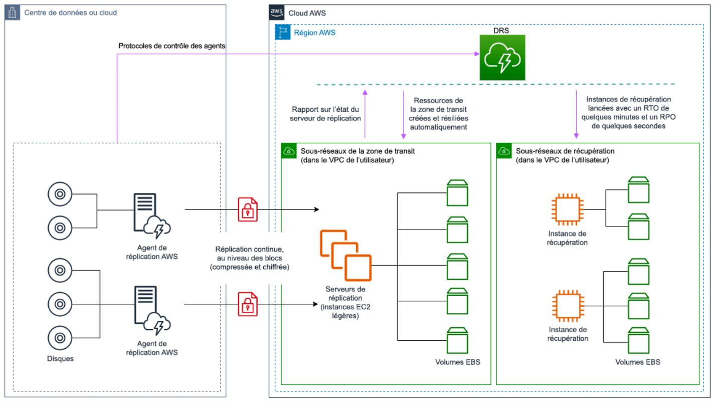
Figure 23 : architecture AWS Elastic Disaster Recovery
