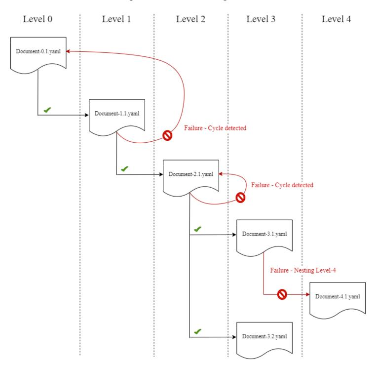
If a component document tries to run itself, or to run any of the component documents that are higher up in the current chain of execution, the execution fails.
