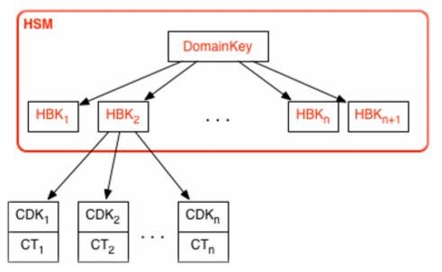
You can make requests through AWS KMS to use your KMS keys to directly protect information or request additional HSM-generated keys that are protected under your KMS key. These keys are called customer data keys, or CDKs. CDKs can be returned encrypted as ciphertext (CT), in plaintext, or both. All objects encrypted under a KMS key (either customer-supplied data or HSM-generated keys) can be decrypted only on an HSM via a call through AWS KMS.
