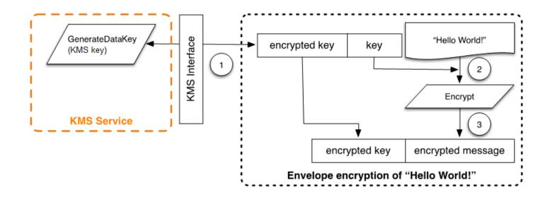
The envelope-encrypted message can be decrypted using the decrypt functionality to obtain the originally encrypted message.
