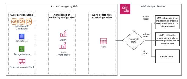
After your resources are tagged based on the policy defined using Resource tagger, and alarm definitions are deployed, the following diagram depicts the AMS monitoring architecture.
