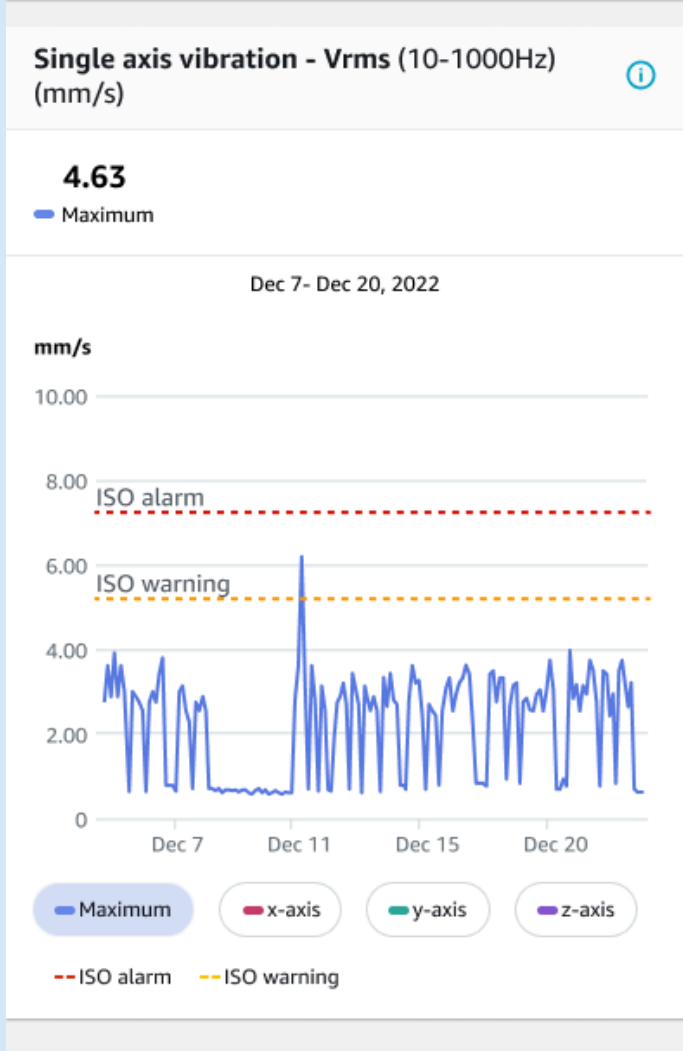
Sensor reading of a healthy asset.
