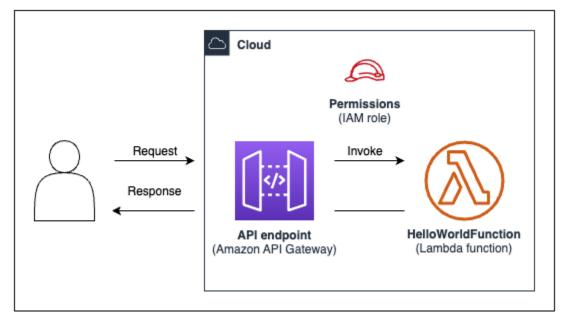
The following diagram shows the components of this application:
