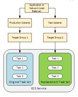
5. Execute any Lambda functions specified in the AfterAllowTestTraffic hook in the AppSpec file. Lambda functions can validate the deployment using the test traffic. For example, a Lambda function can serve traffic to the test listener and track metrics from the replacement task set. If rollbacks are configured, you can configure a CloudWatch alarm that triggers a rollback when the validation test in your Lambda function fails.
