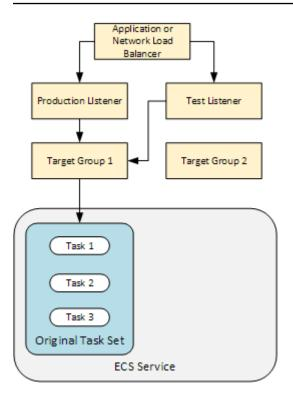
When the deployment starts, the deployment lifecycle events start to execute one at a time. Some lifecycle events are hooks that only execute Lambda functions specified in the AppSpec file. The deployment lifecycle events in the following table are listed in the order they execute. For more information, see AppSpec 'hooks' section for an Amazon ECS deployment.
