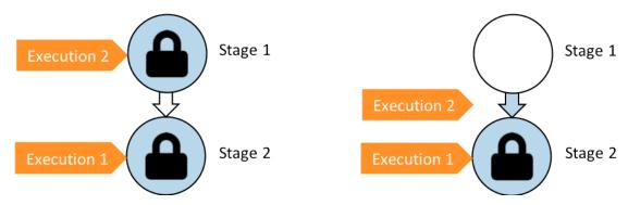
**Before:** Stage 2 is locked as Execution 1 enters. **After:** Execution 2 exits Stage 1 and waits between stages.
