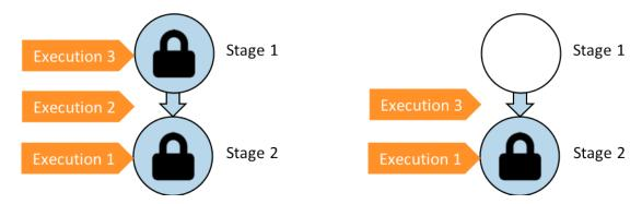
**Before:** execution 2 waits between stages while execution 3 enters stage 1. **after:** execution 3 exits stage 1. execution 2 is superseded by execution 3.
