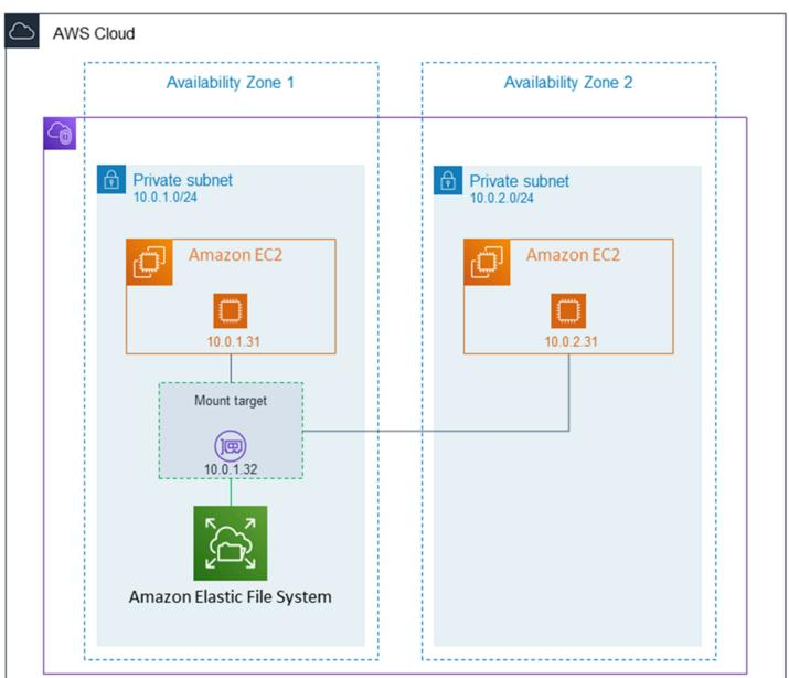
In this illustration, the VPC has two Availability Zones, each with one subnet. Because the file system type is One Zone, it can only have a single mount target. For better performance and cost,
