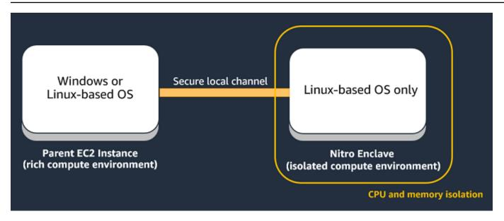
This also means that you must use a Linux-based instance to build your enclave image file (.eif).
