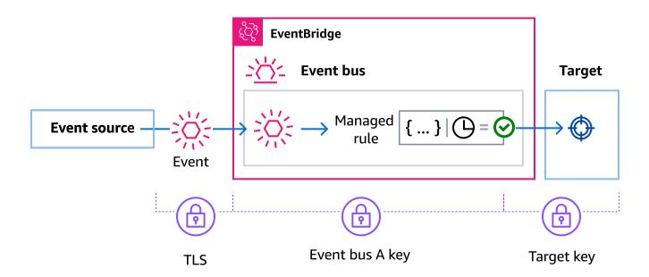
For cases where the rule target is an event bus in another Region, you must provide a <u>multi-Region</u> <u>key</u>. The event bus in the first Region encrypts the event using the customer managed key specified in the managed rule. It then sends the event to the target event bus in the second Region. That event bus must be able to continue to use the customer managed key until it sends the event to its target.
