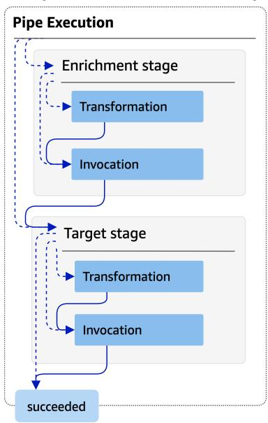
The diagram below presents a detailed view of the pipe execution flow, with all possible execution steps represented. Again, diverging paths are formatted as dotted lines
