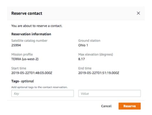
AWS Ground Station will use the configuration data from your mission profile to execute a contact at the specified ground station.
