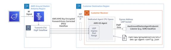
DigIF dataflow from an AWS Ground Station Antenna Region to your EC2 instance with your Software-Defined Radio (SDR) or similar listener.
