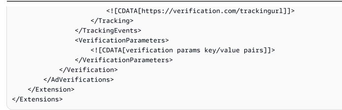
MediaTailor extracts the AdVerifications data from the <Extensions> node and places it into the adVerifications array in the client-side tracking response.
