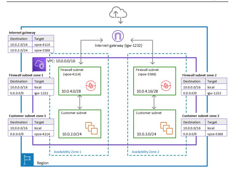
In the preceding figure, the route tables enforce similar traffic flows to the single Availability Zone model, with the primary difference being the splitting of incoming traffic by the internet gateway, to accommodate the two different customer subnets:
