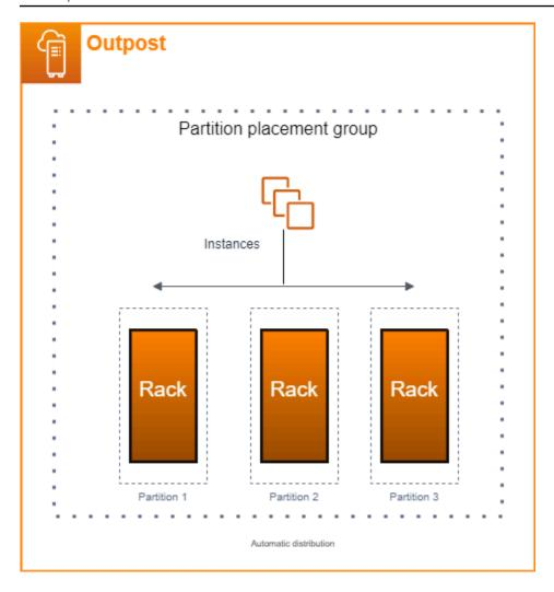
You can also deploy instances to target partitions. The following illustration shows a partition placement group with targeted distribution.
