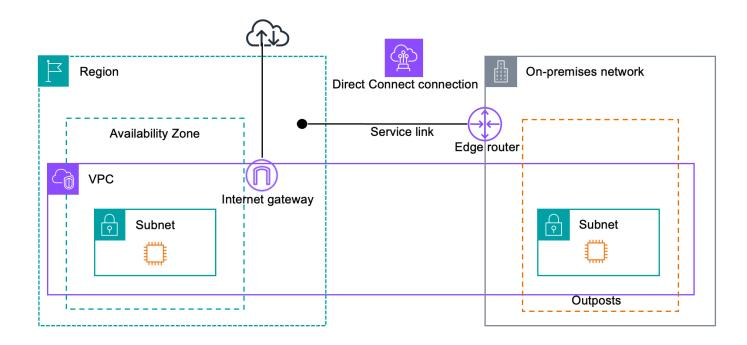
If you are using a stateful firewall with your internet connection to limit connectivity from the public internet to the service link VLAN, you can block all inbound connections that initiate from the internet. This is because the service link VPN initiates only from the Outpost to the Region, not from the Region to the Outpost.
