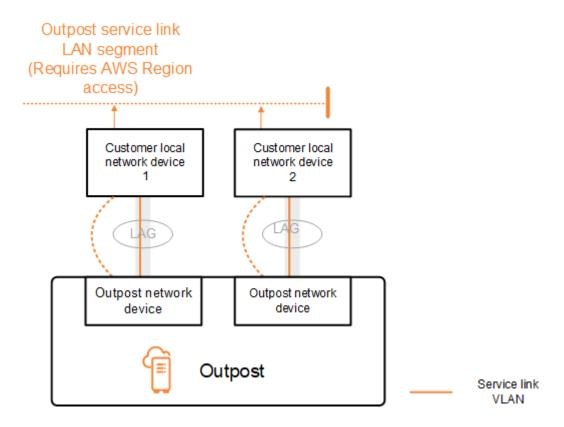
The Outpost establishes an external BGP peering session over the service link VLAN using the following process:
