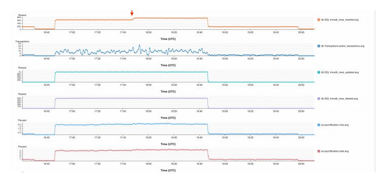
There is no significant change in the CPU utilization with pt-archiver running in parallel, which infers that pt-archiver doesn't impact OLTP queries while running.
