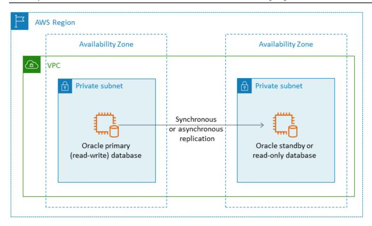
You can also use Oracle Data Guard or Oracle Active Data Guard to configure high availability and disaster recovery across multiple AWS Regions, using Oracle Database on Amazon EC2 for your primary database and standby database, as illustrated in the following diagram.
