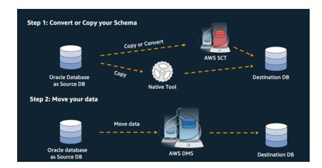
AWS DMS handles all required data type conversions automatically during migration. The source database can be located in your own premises outside AWS, it can be a database that's running on an EC2 instance, or it can be an Amazon RDS database (see <a href="Sources for data migration">Sources for data migration</a> in the AWS DMS documentation). The target can be a database in Amazon EC2, Amazon RDS, or Amazon Aurora.
