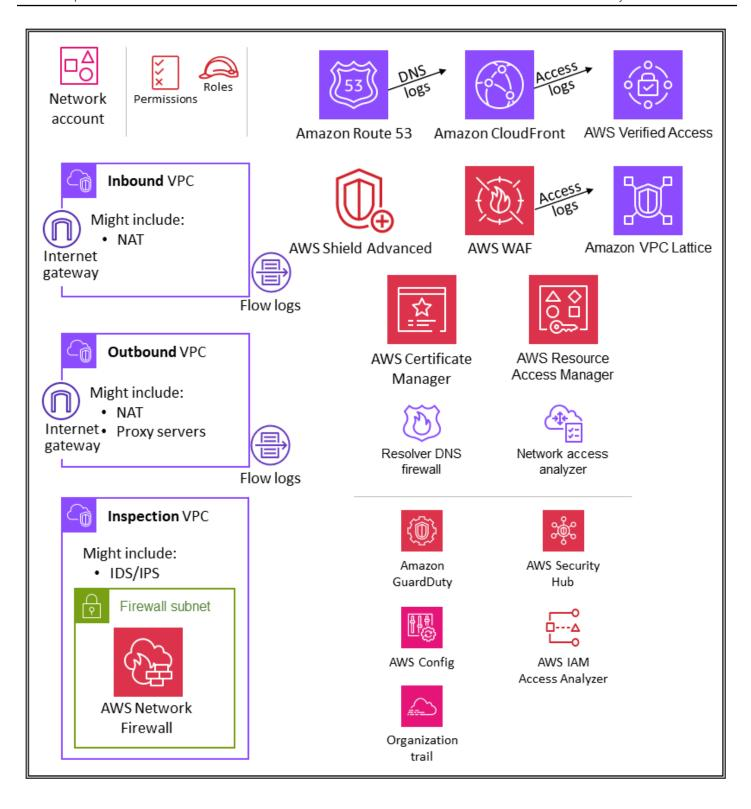
The Network account manages the gateway between your application and the broader internet. It is important to protect that two-way interface. The Network account isolates the networking services, configuration, and operation from the individual application workloads, security, and other infrastructure. This arrangement not only limits connectivity, permissions, and data flow, but
