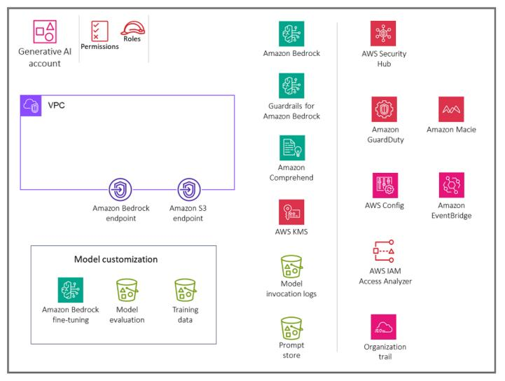
The Generative AI account includes services required for customizing a model along with a suite of required security services to implement security guardrails and centralized security governance. You should create Amazon S3 gateway endpoints for the training data and evaluation buckets in Amazon S3 that a private VPC environment is configured to access to allow for private model customization.
