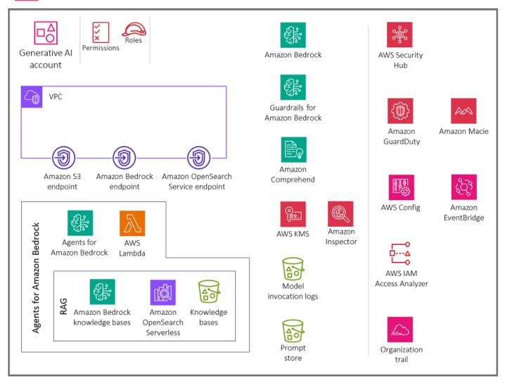
The Generative AI account includes services that are required for calling AWS Lambda parser functions for agent workflows, using Amazon Bedrock knowledge bases as part of agent workflows, and storing conversations for users. It also includes a suite of required security services to implement security guardrails and centralized security governance.
