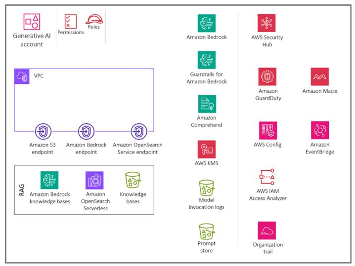
The Generative AI account includes services that are required for storing embeddings in a vector database, storing conversations for users, and maintaining a prompt store along with a suite of required security services to implement security guardrails and centralized security governance. You should create Amazon S3 gateway endpoints for the model invocation logs, prompt store, and knowledge base data source buckets in Amazon S3 that the VPC environment is configured to
