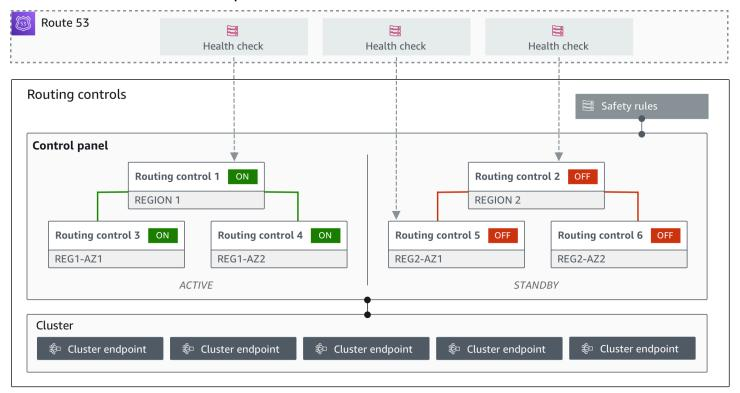
The following are components of the routing control feature in Route 53 ARC.
