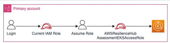
The following conceptual diagram shows how AWS Resilience Hub accesses Amazon EKS clusters deployed on a secondary account when the application is configured to use the current IAM user permissions.
