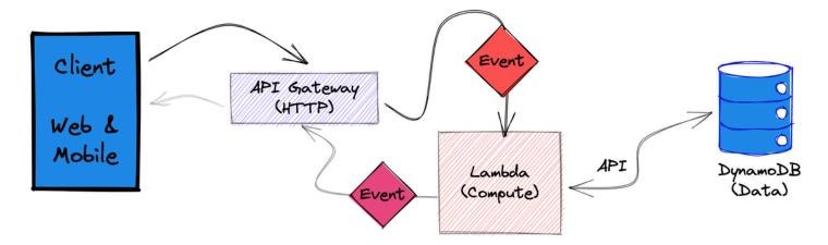
Many traditional systems are designed to run periodically and process batches of transactions that have built up over time. For example, a banking application may run every hour to process ATM transactions into central ledgers. In Lambda-based applications, the custom processing should be triggered by every event, allowing the service to scale up concurrency as needed, to provide near-real time processing of transactions.
