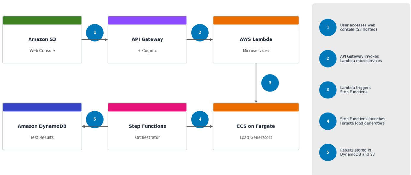
Distributed Load Testing on AWS — Architecture
