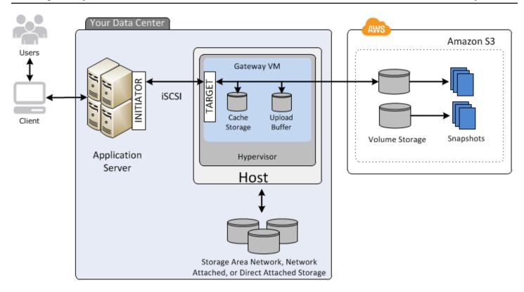
After you install the Storage Gateway software appliance—the VM—on a host in your data center and activate it, you use the AWS Management Console to provision storage volumes backed by Amazon S3. You can also provision storage volumes programmatically using the Storage Gateway API or the AWS SDK libraries. You then mount these storage volumes to your on-premises application servers as iSCSI devices.
