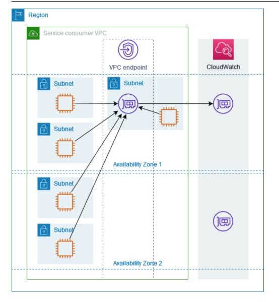
The following diagram shows a VPC endpoint for Amazon CloudWatch with endpoint network interfaces in two Availability Zones. When any resource in any subnet in the VPC accesses Amazon CloudWatch by using its public endpoint, we select a healthy endpoint network interface, using the round robin algorithm to alternate between them. We then resolve the traffic to the IP address of the selected endpoint network interface.
