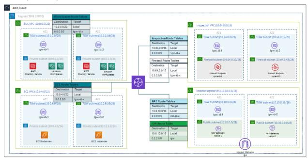
Figure 22: Sample architecture using Transit Gateway attachments
