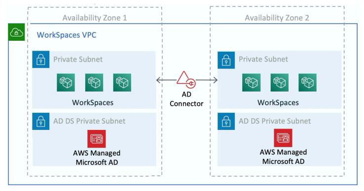
Figure 13: AD DS network separation
