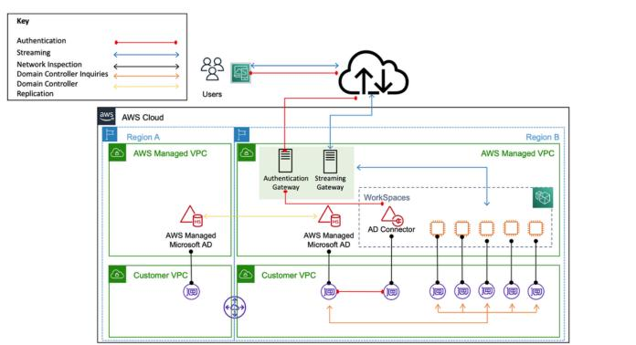
Figure 12: Sample architecture for registering a replicated MAD region to a WorkSpace
