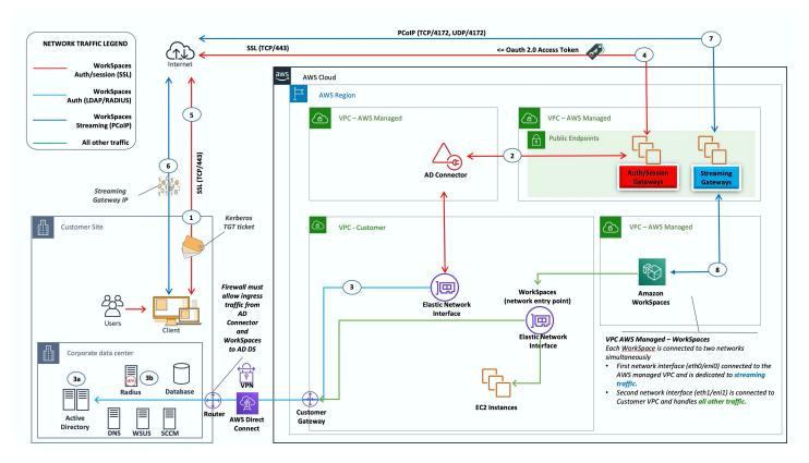
Figure 5: AD Connector to on-premises Active Directory
