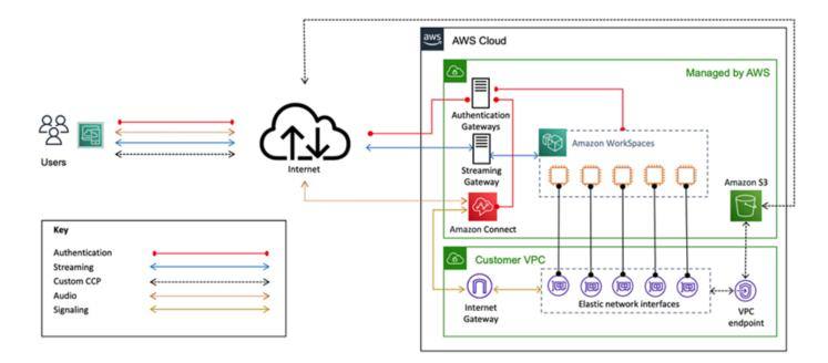
Figure 26 — Amazon Connect and WorkSpaces Architecture Diagram
