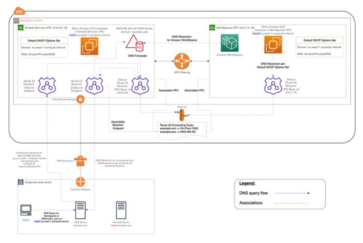
Figure 2: WorkSpaces DNS resolution example with Route 53 endpoints
