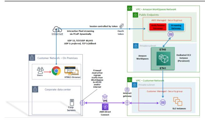
Figure 20: Web access client architecture
