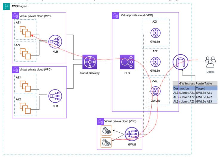
Centralized ingress traffic inspection using firewall appliances with Gateway Load Balancer
