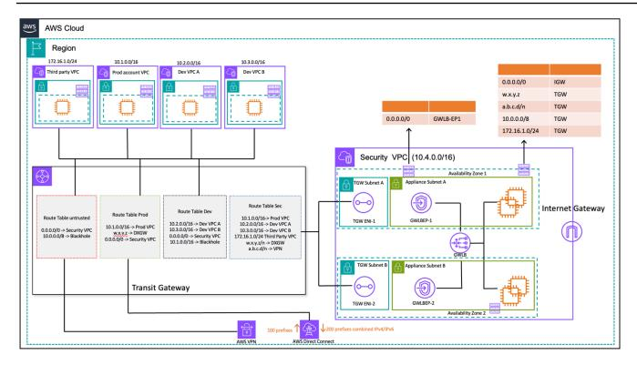
VPC-to-VPC and on-premises-to-VPC traffic inspection using Transit Gateway and AWS Gateway Load Balancer (route table design)
