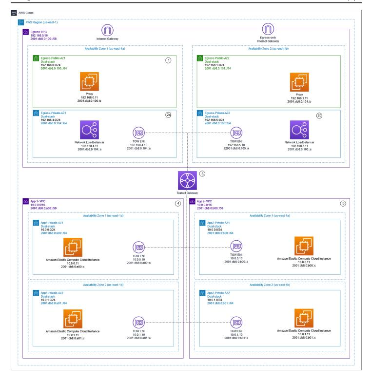
Centralized IPv4 and IPv6 egress using proxy instances and Network Load Balancer
