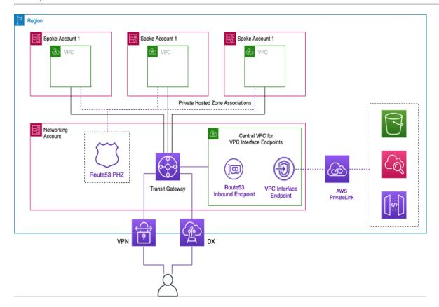
Centralizing interface VPC endpoints
