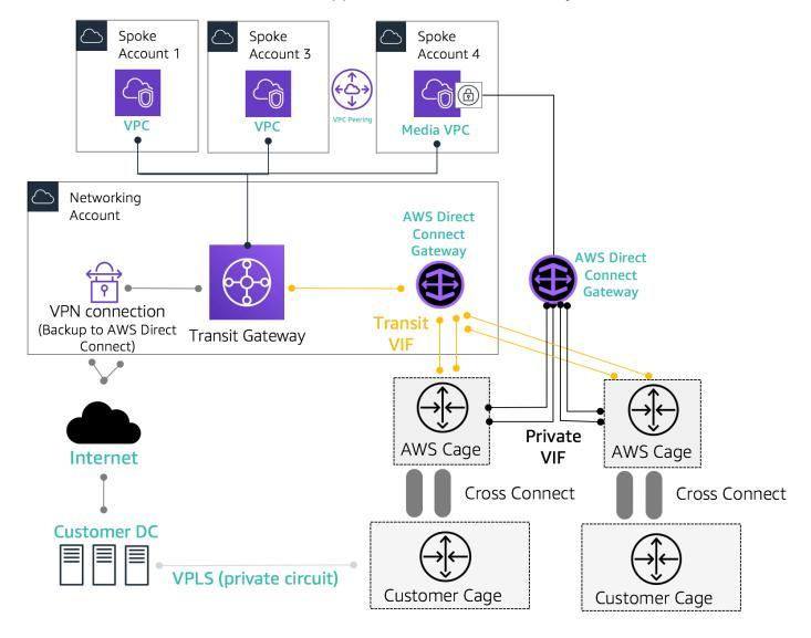
Sample reference architecture for hybrid connectivity
