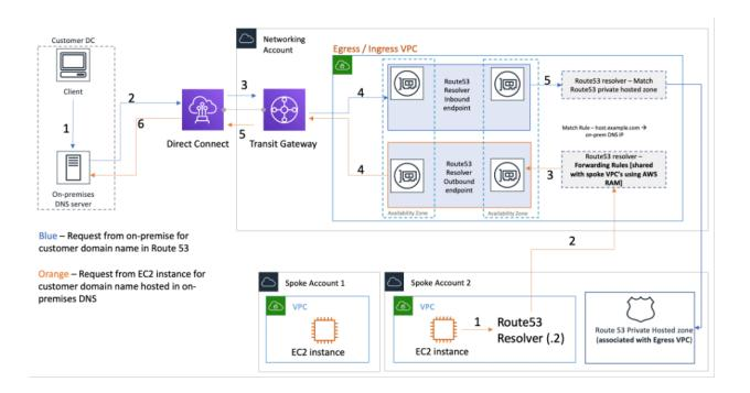
Centralizing Route 53 Resolver endpoints in ingress/egress VPC
