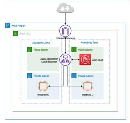
Centralized inbound traffic inspection using AWS WAF
