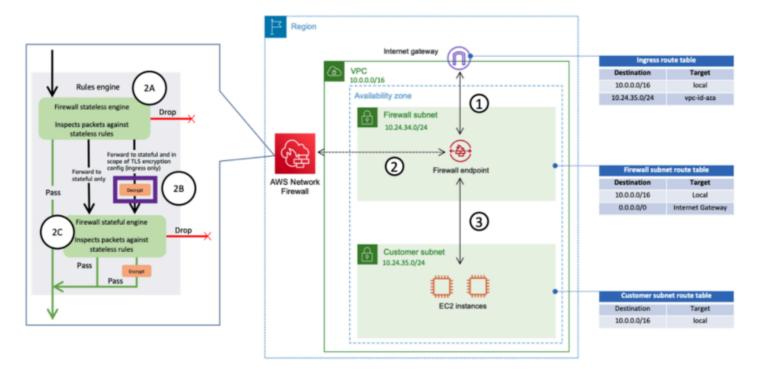
Ingress traffic inspection using Network Firewall with DPI
