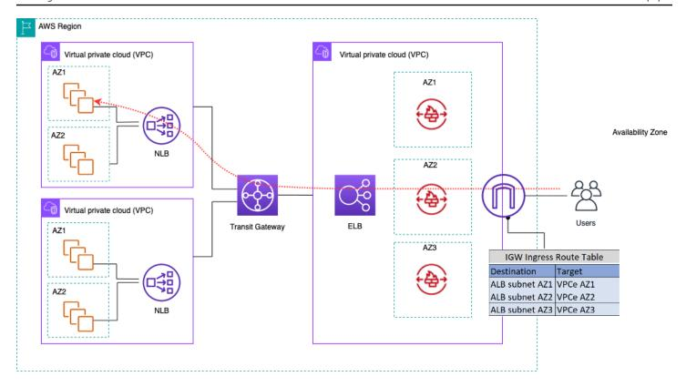
Ingress traffic inspection using AWS Network Firewall
