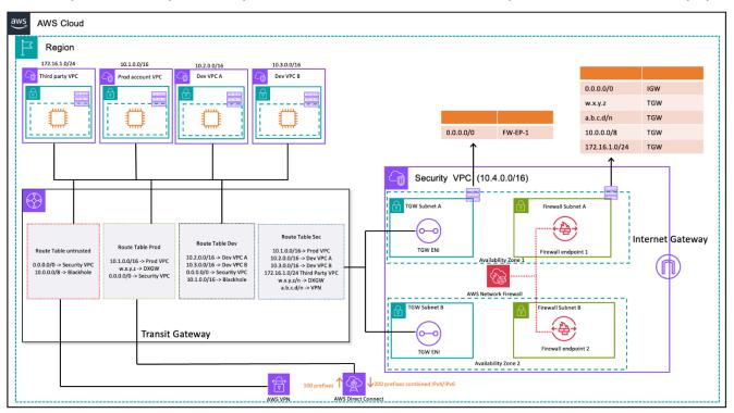
VPC-to-VPC and on-premises to VPC traffic inspection using Transit Gateway and AWS Network Firewall (route table design)
