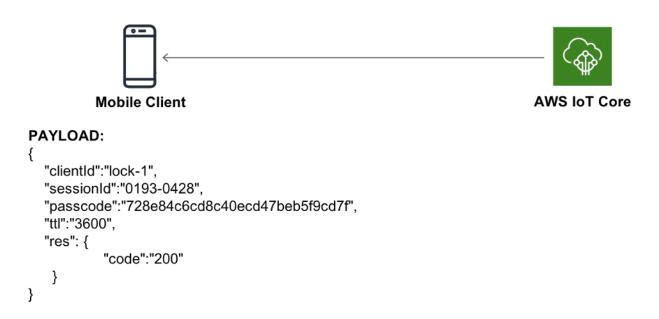
Command response sent from AWS IoT Core to mobile client
