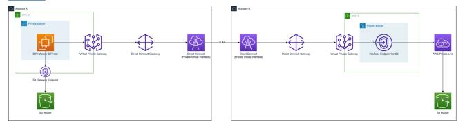
DTH worker nodes running on EC2 transfer data from bucket in one AWS account to bucket in another AWS account.
