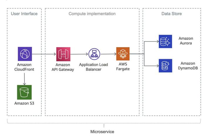
Figure 5: Serverless microservice using AWS Fargate
