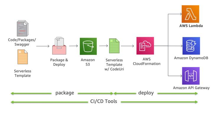
Figure 2: AWS Serverless Application Model (AWS SAM)
