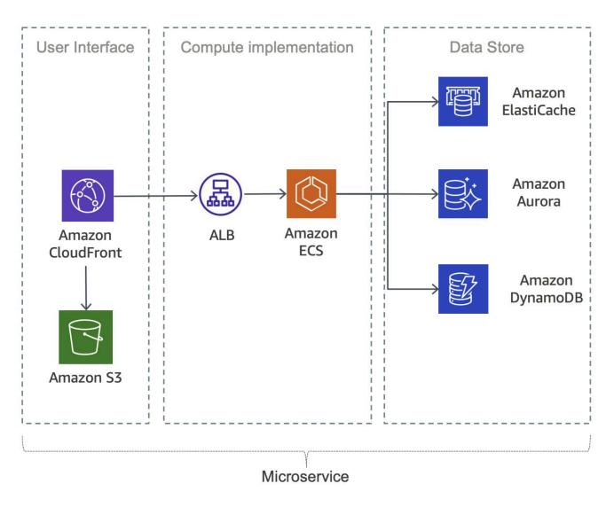
Figure 1: Typical microservices application on AWS
