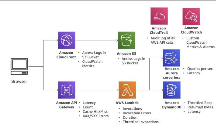
Figure 10: A serverless architecture with monitoring components
