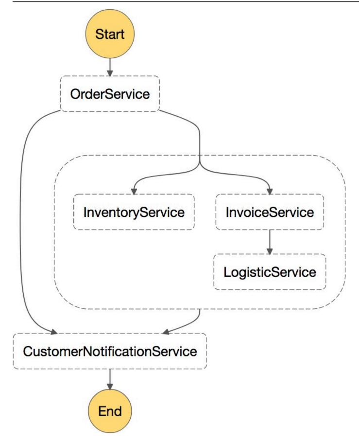
*Figure 9: An example of a microservices workflow with parallel and sequential steps invoked by AWS Step Functions*
